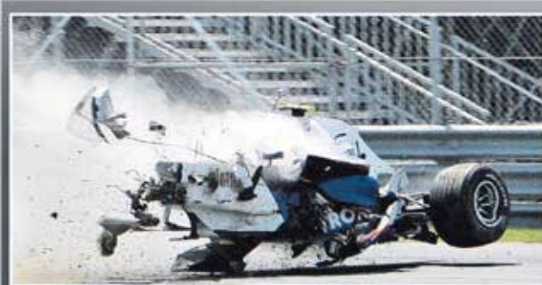
Design of the car must also include an impact-absorbing structure at the rear, behind the gearbox
